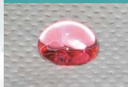
A drop of water on a superhydrophobic nonwoven.
